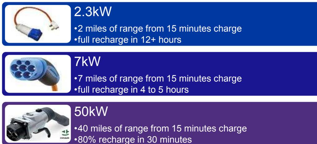
Figure 1 - Charging speed and typical increases in range from a 15 minute charge. Actual mileage gains and time taken to charge will vary by vehicle model.
