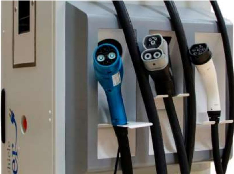
Figure 6 - Rapid chargepoint incorporating all three protocols.
