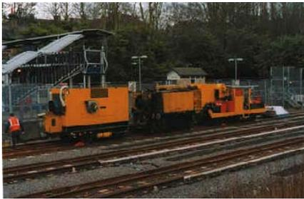
Rail grinding to restore rail profiles continues to be a successful noise reduction measure. 3 sites have been completed this year – Victoria-Brixton, Highbury-Kings Cross and Highbury-Seven Sisters. Other changes such as lubrication of curved sections, train speed restrictions in sensitive areas and better line-side vegetation management are also helping.
