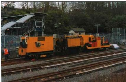
Rail grinding to restore rail profiles continues to be a successful noise reduction measure. Last year, over 20 km of track was reground or replaced. Other engineering practices, such as lubrication of curved sections, train speed restrictions in sensitive areas and better line-side vegetation management are also helping to reduce noise levels.
