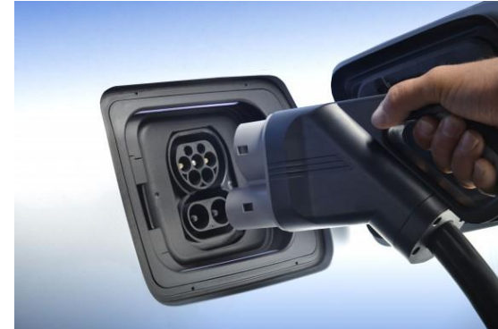
Figure 1 the CCS connector which may become a mandatory requirement of all new charging stations in Germany
