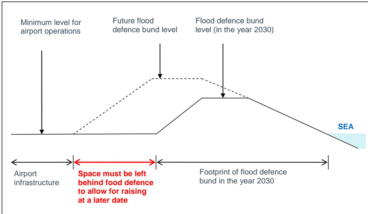
**Figure 3-1 Safeguarding for future reinforcement of flood defence bund**
