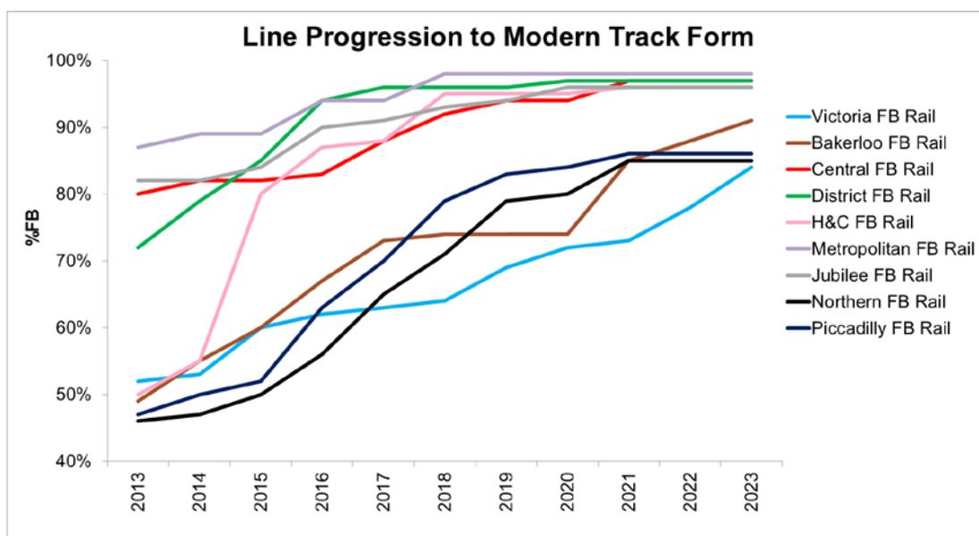
Figure 1: Progression to modern track form ie Flat-Bottom (FB) Rail, by line.
