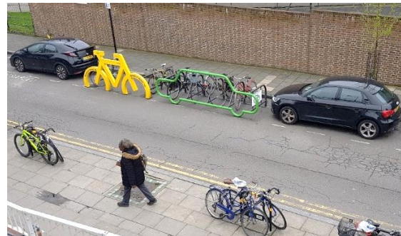
Figure 1: Cycle parking installed on space taken from car parking bay. In order to ensure maximum space for social distancing on the footway during coronavirus-recovery, access to cycle parking should ideally be from the carriageway, rather than from the footway.
