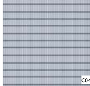
C04: Blue woven mesh stainless steel panel in vibration/brushed finish. Panel fixed using proprietary cladding system with 20mm shadow gap to all sides.
