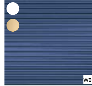
W07: Blue profiled stainless steel panel in vibration/brushed finish. Panel fixed using proprietary cladding system with 10mm shadow gap to all sides.
