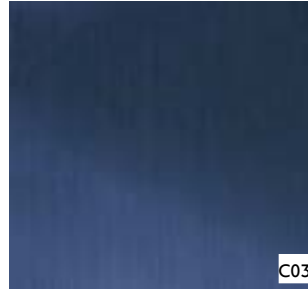
C03: Blue stainless steel panel in vibration/brushed finish. Panel fixed using proprietary cladding system with 20mm shadow gap to all sides.
