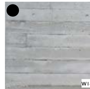
W14: In-situ concrete with 20mm shallow gap recess to all module edges. Concrete to be cast in 600mm wide module pattern to match wall panels.
