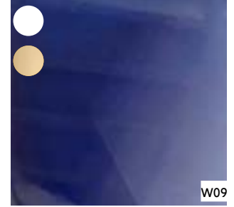
W09: Blue back painted glazed panel, secret fixed using proprietary cladding system.
