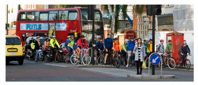
The available lane widths and position of the central refuge prevents both cyclists and motorcyclists from filtering on the approach to the traffic signals.
