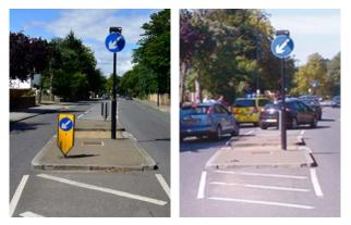
These two pictures show the same refuge, one with a low-level keep left bollard and the other where the bollard is missing. The missing bollard increases the risk of a vehicle striking the refuge, particularly at night or in bad weather.
