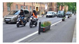
Although more difficult to see than up-right bollards, the low level 'Zicla' separators are positioned well away from the general traffic lane and do not cause a problem for motorcyclists.
