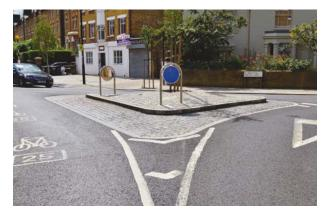
The cobbled overrun area in this picture is in an area where motorcycles may be leant over, and could be slippery when wet. Also the white lines may guide motorcycles into the cobbled area at night, rather than around it.
