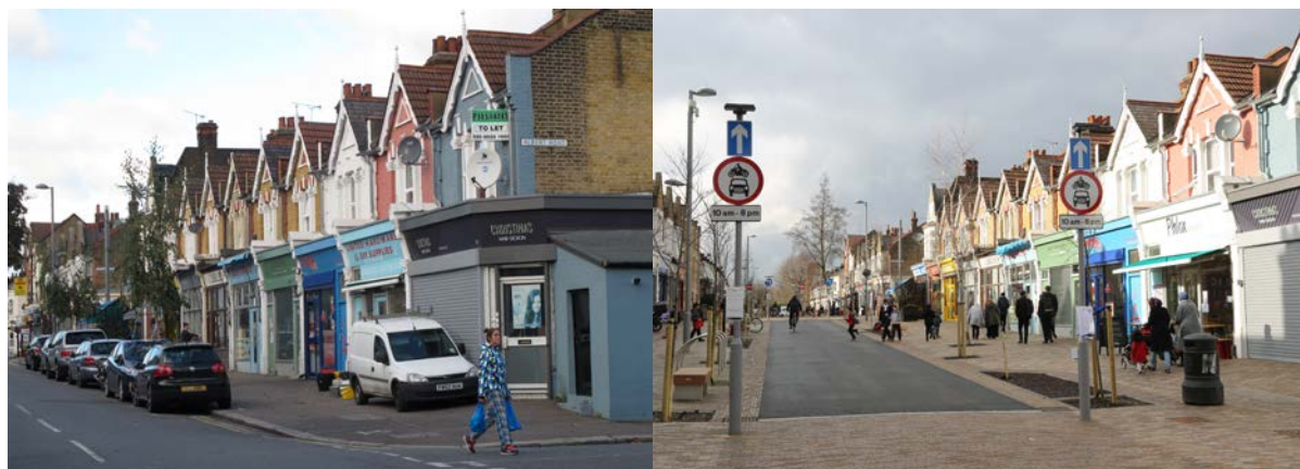
Figure 5.25 Francis Road, Leyton – before and after the ‘modal filtering’ scheme which restricts vehicle access, and provides wider pavements and cycle stands.
