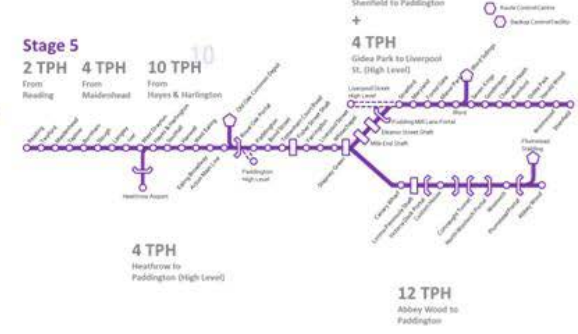
Central Section service connected to Great Western surface section. Passenger services operational from Maidenhead and Heathrow to Shenfield and Abbey Wood
