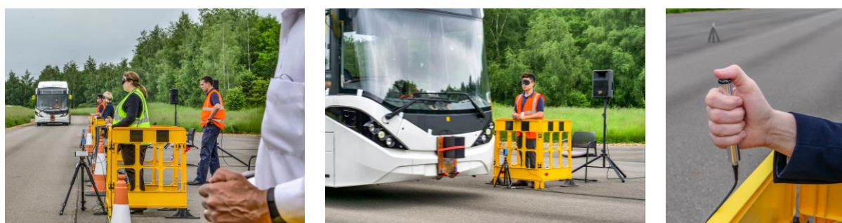
Figure 6-2: Test set up showing bus approaching participants (left), bus with rudimentary added sound on front level with participant and background noise speaker (middle), participant holding trigger switch (right)
