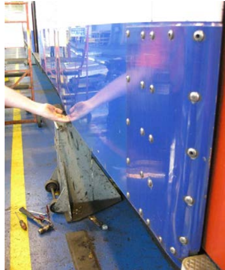
Failed car body side stiffener bracket
