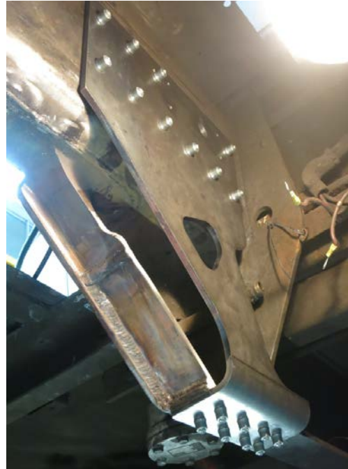
Swan neck repair (with bracket)
