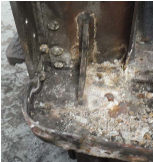
Car body corner post corrosion
