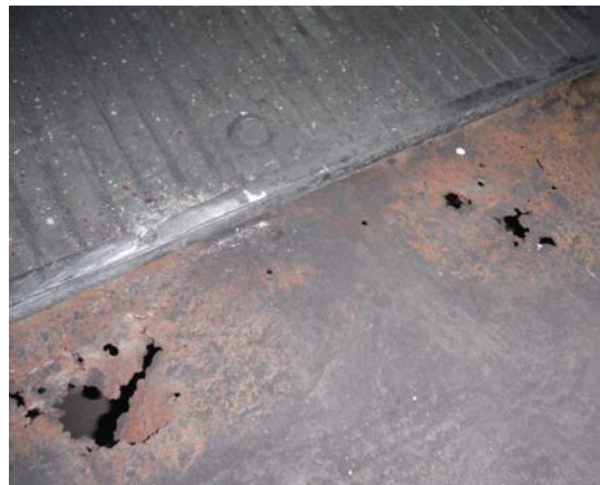
Saloon floor plate corrosion
