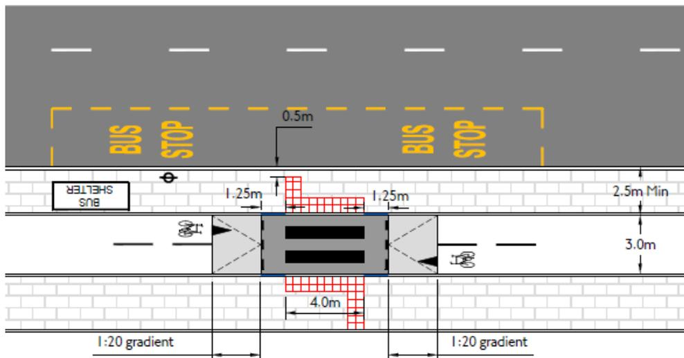
In both layouts, the crossing will be located such that the passenger will turn left when exiting the bus to locate the crossing, when one bus is at the stop, and it is stopped in the correct place. When walking from the footway to the bus stop, the passenger turns left to locate the bus stop flag, in the standard layout.
