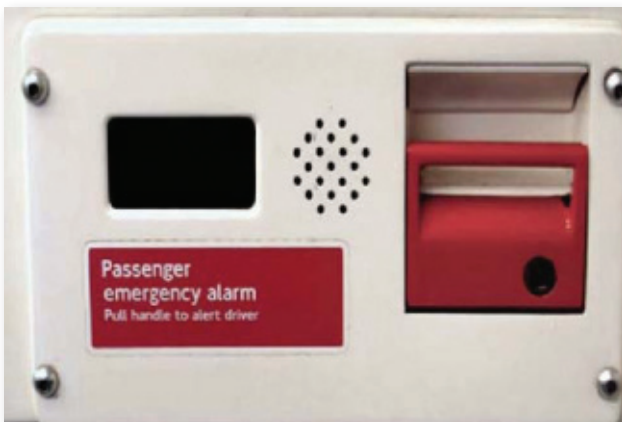
Underground train passenger alarm point
