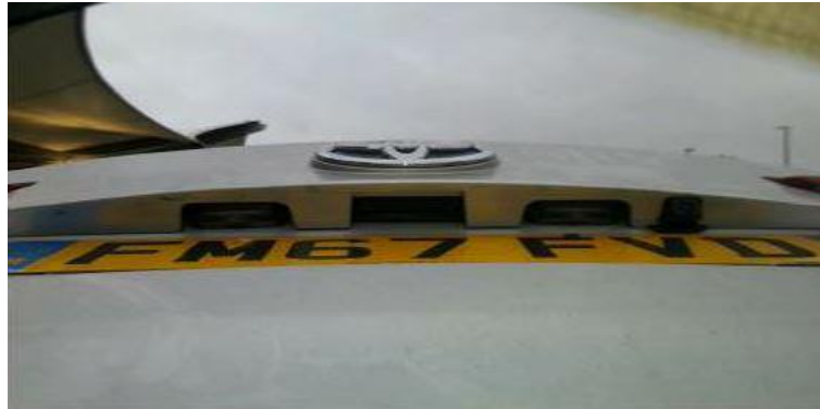
Picture 2 – faulty/no VRM lights
