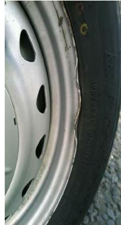
Picture 5 – damaged wheel rim
