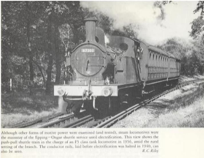
Although other forms of motive power were examined (and tested), steam locomotives were the mainstay of the Epping–Ongar shuttle service until electrification. This view shows the push-pull shuttle train in the charge of an F5 class tank locomotive in 1956, amid the rural setting of the branch. The conductor rails, laid before electrification was halted in 1940, can also be seen.
