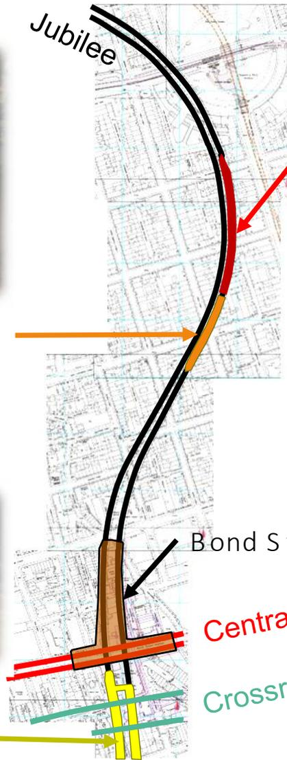
“BS BS” Baker Street to Bond Street deterioration of 200 metres of concrete lined
