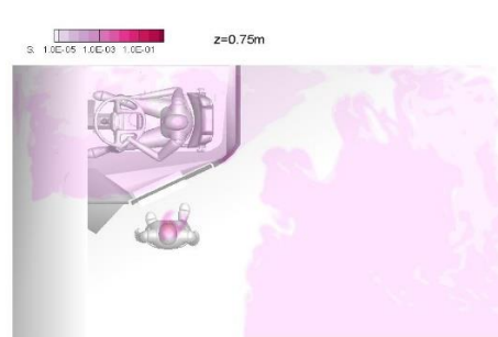
Figure 2: Isosurface of 0.1% droplet concentration after 60s. Left: Oblique view from behind the passenger, Right: View from above the passenger
