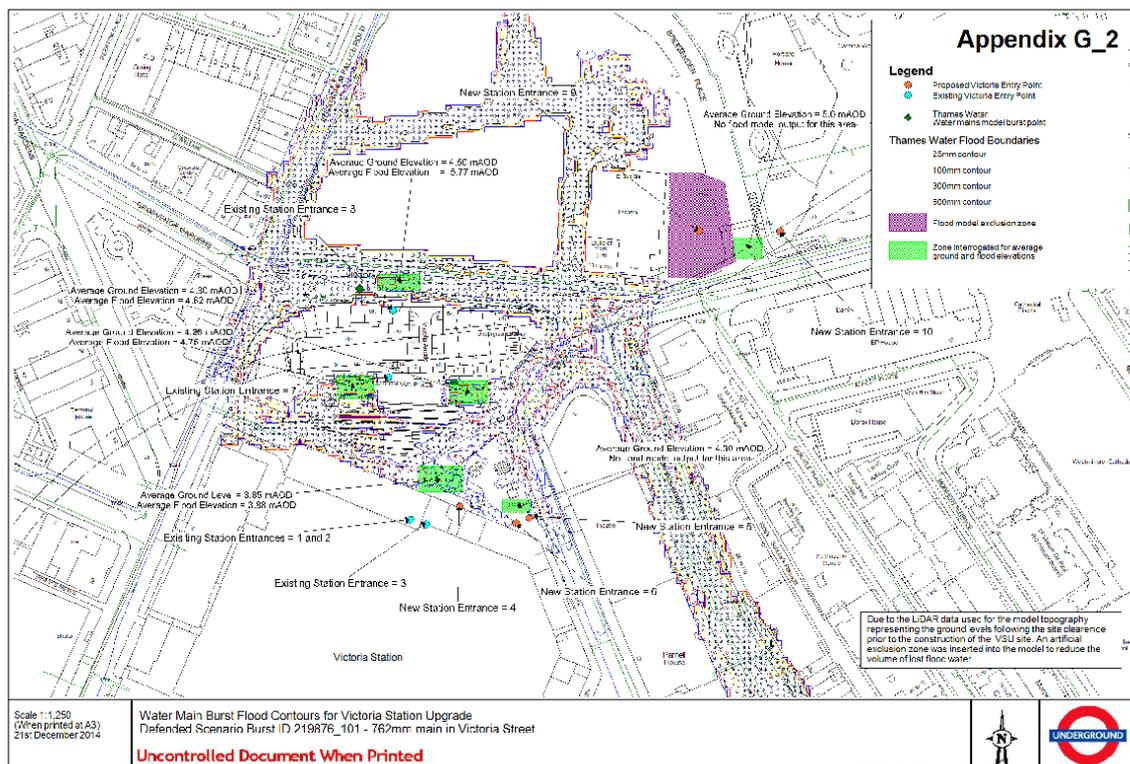
**Figure x – Burst water mains hydraulic model output**
